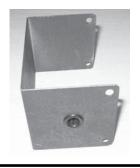
23) Run the other end of the ground wire and DC spark generator wires through the bushing on the heat shield.
